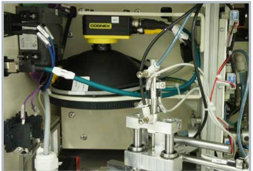
*A camera image processing system in one of our machines, with a large dome illumination preventing glare on shiny surfaces*
