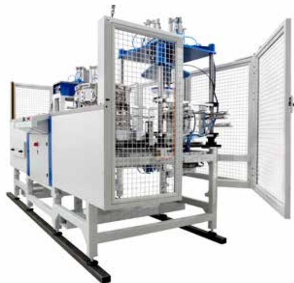
*Cast leakage inspection equipment*
