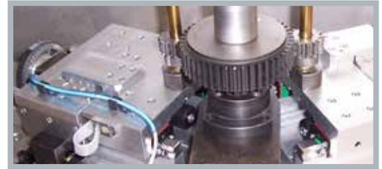
*The submicrometer measurement tool of a cogwheel inspection equipment*
